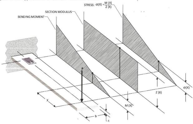
For a parallel-sided beam, as illustrated in the preceding sketch the axial stress on the beam surface is proportional to the bending moment, and is expressed by:
