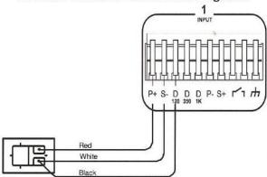
**D4 Strain Indicator Connection Diagrams**
