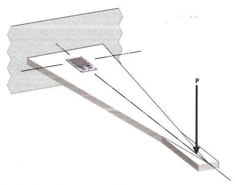
Note that the sides of the beam in the constant-stress section must still converge toward the point of load application to satisfy Eq. (7) over this region.
